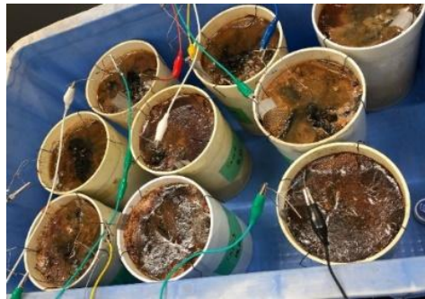
Fig. 1 Floating food waste particles into the cathode chamber
